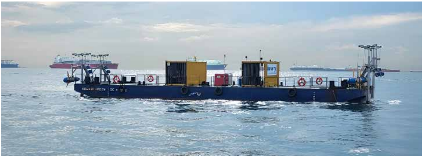
Figure 1: Floating barge with turbines installed at both ends for generating electricity.
