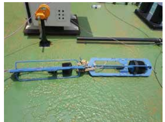
Figure 4: Single point Doppler Current Sensor (DCS) and Doppler Current Profiler Sensor (DCPS) housed in individual mooring protective frames to measure current velocities and direction at near water surface and water column.
