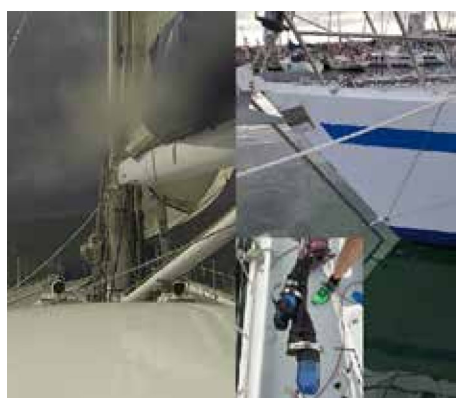
Fig. 2: Sensors to measure oxygen, salinity, temp, pH and pCO 2 were installed on a stainless steel pole that was attached in the bow of S/Y Hrimfare. Data from the sensors and the position from the boats GPS were logged every 20sec by a SmartGuard sensor hub. The entire installation took about 2 hours.
