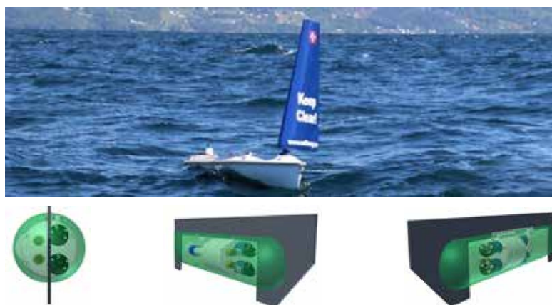
Fig. 3: SailBuoy with Aanderaa antifouling protected sensor package placed in the keel bulb
