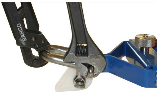
Figure 6-4 Fasten shackle in frame. Tighten thoroughly.
