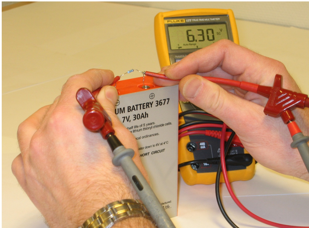
Figure 6-19 Use a 100 \Omega resistor up to 6.3 V to rejuvenate the battery. Note! Illustration shown with older Lithium batteries; today's batteries have connection pins at the side, not on top.
