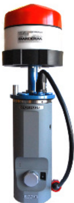
Figure 1-1 An example of the SeaGuardII Platform with DCPS and oxygen sensors mounted on the top-end plate and external cable for real time communication
