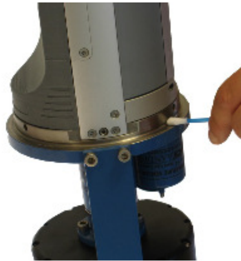
Figure 8-2 Clean O-ring seating; instrument up-side-down.
