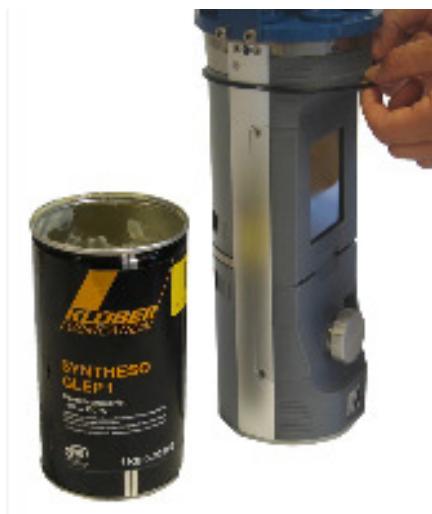
Figure 8-5 Lubricate O-rings with grease. (Klüber Lubrication Syntheso Glep 1 or similar synthetic grease).
