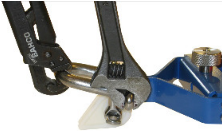
Figure7-3 Fasten shackle in frame. Tighten thoroughly.
