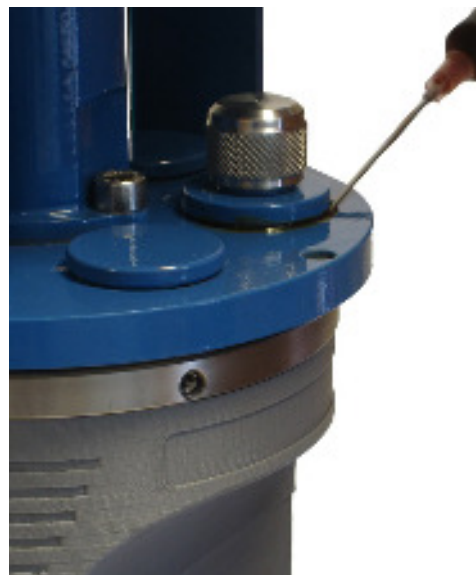
Figure 8-2 Clean O-ring seating; instrument up-side-down.
