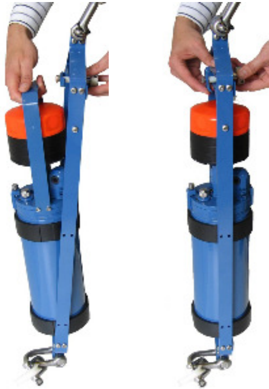
Figure7-6 Mount the instrument into the frame.
