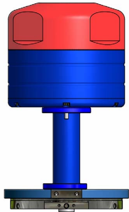
Figure 9-2 Drawing of an ZPulse™ DCS 4520/4930 mounted onto a Stud and Connected to the SeaGuard Top-end Plate.
