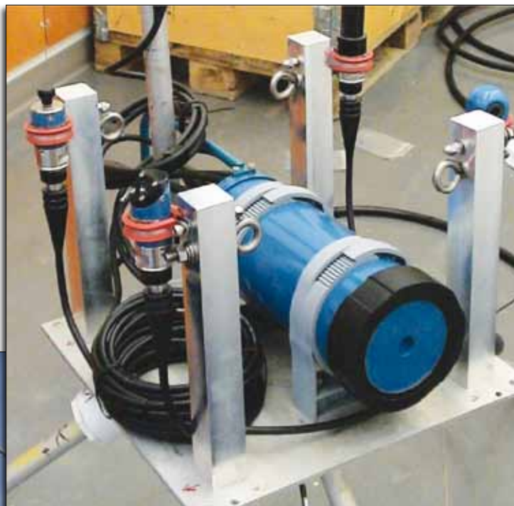
Fig. 1. The UNC HANDI Seaguard logger multi-sensor platform on a stand for deployment on the seafloor. HANDI features two multi-sensor "strings" that can be utilized to place individual sensors near exposed gas hydrates, gas-rich sediments or hydrocarbon gas bubble streams.
