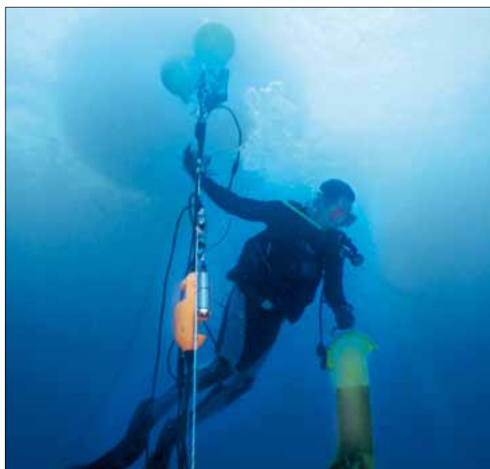
Fig. 5. Diver checking AADI optodes and analog methane sensor (silver cylinder) five meters above bottom under the Aquarius Reef Base Life Support Buoy (Photo by Chris Martens, UNC-Chapel Hill)
