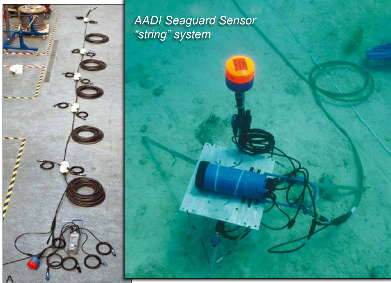
Fig. 3. RANDI features a 170 meter long string with pairs of fast response optodes located every 30 meters along the string (Photos by Tor Arne Hetland, AADI and Chris Martens, UNC-Chapel Hill).
