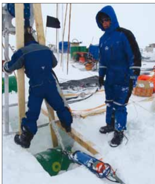
RCM 9 deployed through the hole
