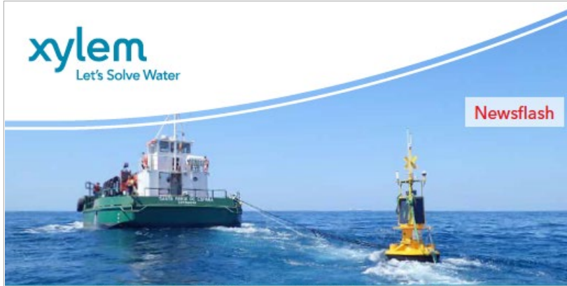
Fig. 1: Deployed SB-138 P buoy equipped with MOTUS wave sensor, DCPS, GMX200 weather sensor, and ATON AIS Type 3
