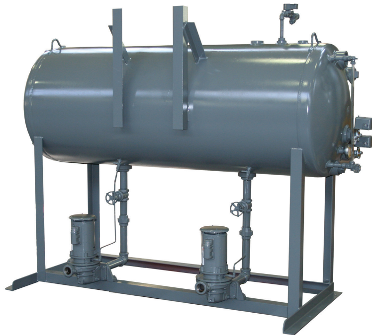
Series CMED Boiler Feed Units for systems with high temperature returns (212°F at sea level), up to 260 gpm and up to 175 psig discharge pressures
