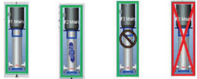
Stand-By Running Off VFD Fail
