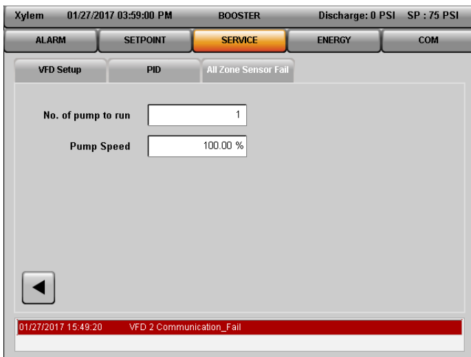
Figure 5.5.13 – All Zone Sensor Fail
