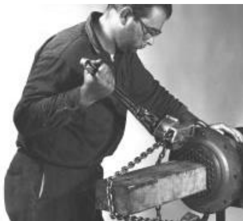
Illustration No. 1 – The method employed to push tube bundle out of shell.
