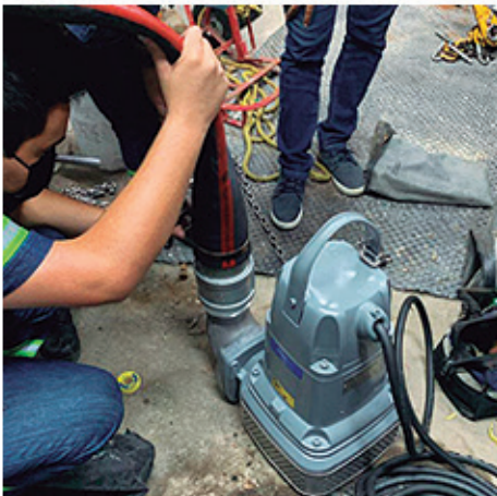
Flygt Bibo Alpha is light and it does not need a crane for its installation.
