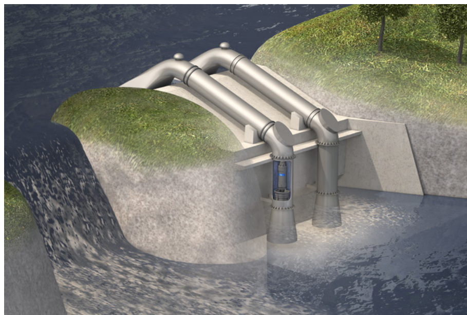
Siphon power station with siphon intake type I.
