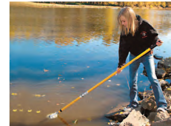
The swing sampler allows for easy sample collection from different angles. Pole extends up to 12 ft.
