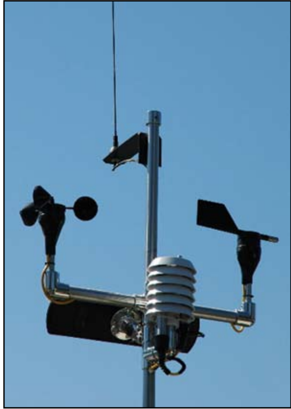
Monitoring weather remotely with Global Water's WE900 Weather Station and SIT65 Satellite Internet Telemetry system.
