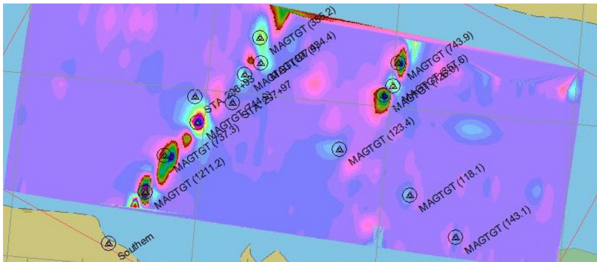
FIGURE 37. Magnetometer Targets Displayed in HYPACK®
