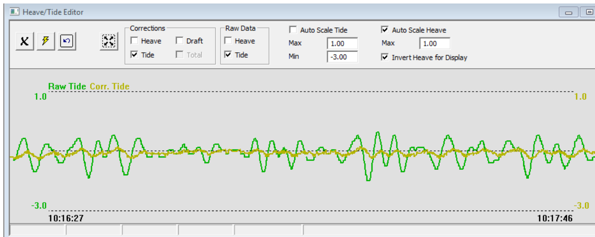
FIGURE 37. Raw Tide (green), Corrected Tide (yellow)—If all were perfect, the corrected tide line would be almost flat.
