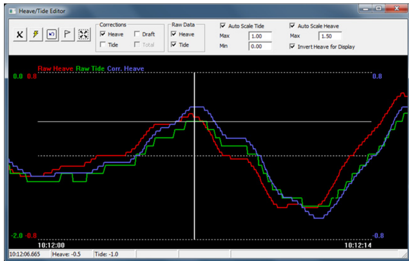
FIGURE 6. Comparing Heave with RTK Tide
