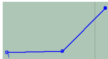
FIGURE 32. Survey Line Extended 45 Survey Units at a Bearing of 45 Degrees
