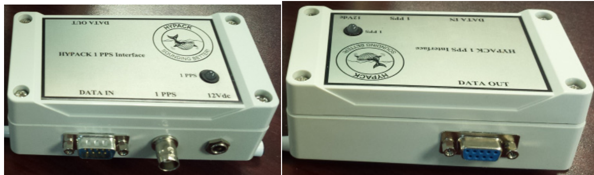
FIGURE 2. 1PPS Box—Input (left): RS232 In from GPS, 1PPS In from GPS, 12V DC In, 1PPS Strobe; Output (right): RS232 Out to PC
