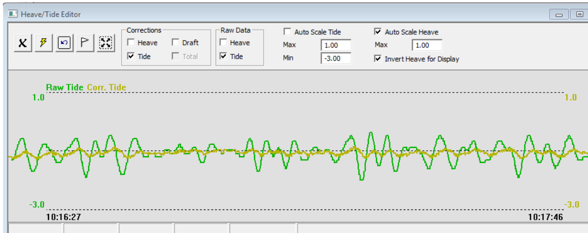
FIGURE 53. Raw Tide (green), Corrected Tide (yellow)—If all were perfect, the corrected tide line would be almost flat.
