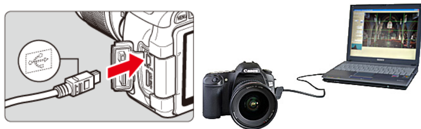
FIGURE 2. Connecting the Canon DSLR Camera via USB to the HYPACK Computer.
