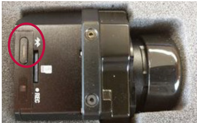
FIGURE 7. Starting the Bluetooth Connection on the Camera
