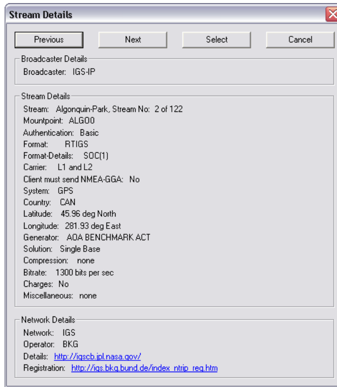
FIGURE 2. Details of GNSS Internet Radio Stream
