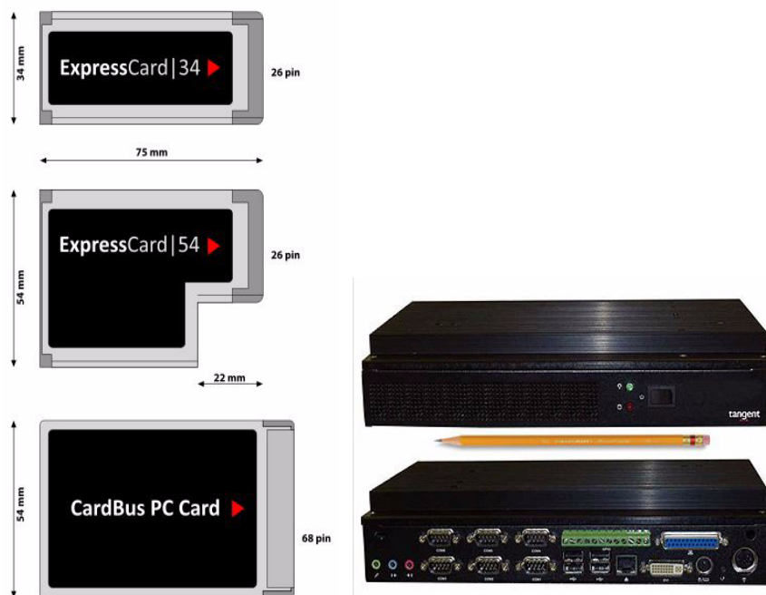
FIGURE 1. Express Cards and CardBus (left), Tangent PC (right)
