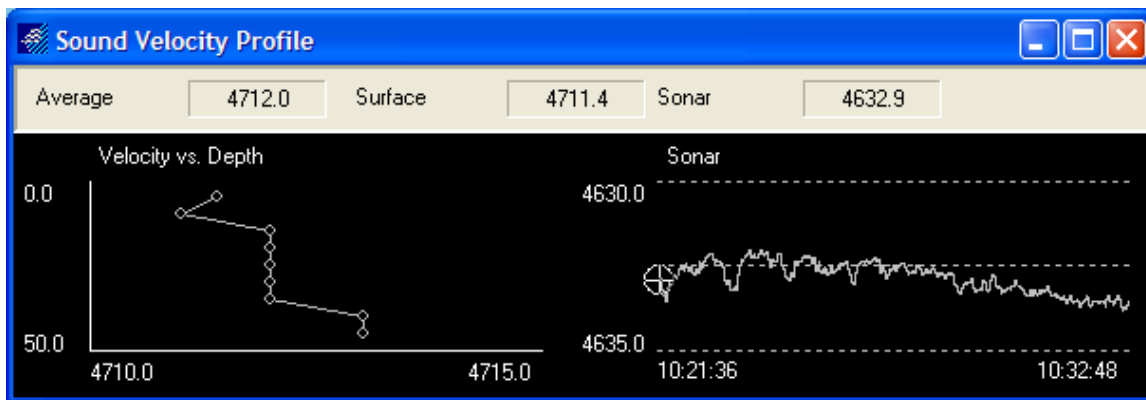
FIGURE 2. Sound Velocity Profile (left) and at the Sonar Head (right)
