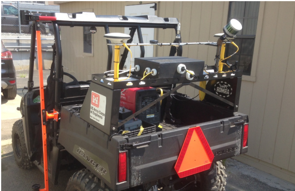
FIGURE 2. New York Corps of Engineers' Velodyne System
