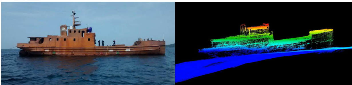
FIGURE 1. ARC Quindío, former Hydrographic Ship used by the Colombian Navy that was sunk nearby Cartagena. On the right a picture of when it was sunk (left) and an image from multibeam data collected and processed with HYPACK®.(right)
