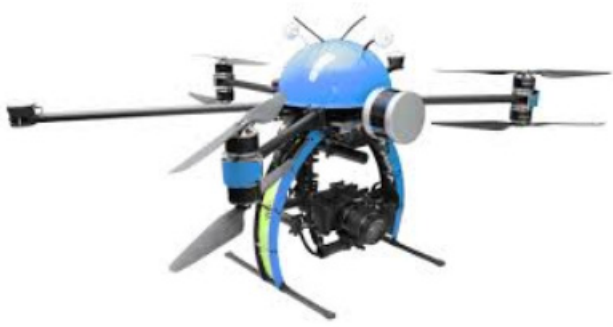
FIGURE 3. NEXUS drone system with the VLP-16 scanner at front pointing downward. This orientation gives 360 degree coverage side to side and +/- 15 degree coverage fore and aft (16 beams at 2 degree spacing).
