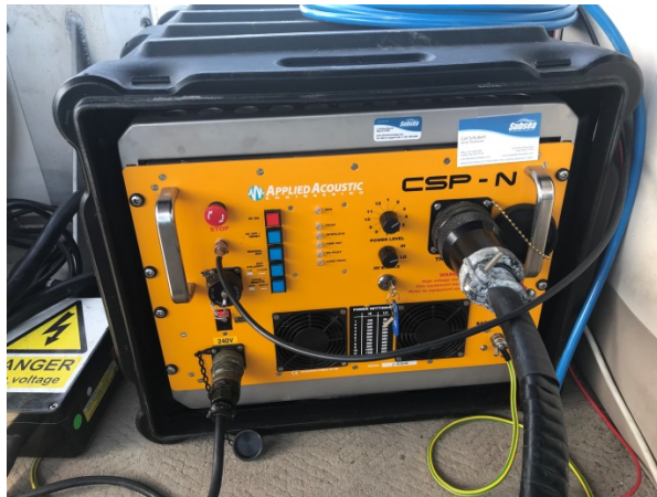
FIGURE 3. Repairs being made to the boomer power supply. Caution – high voltage!
