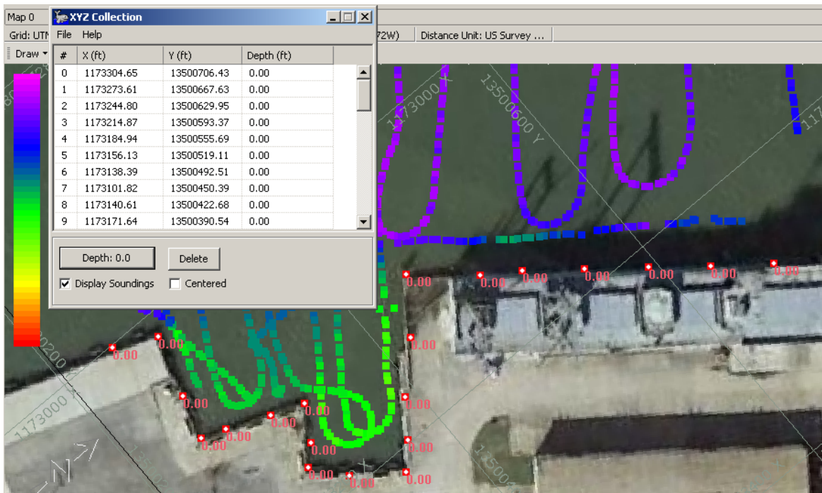
FIGURE 3. Showing Sounding Data and Targets Overlay on the GeoTif Chart Created Using the Image Geo Reference Program
