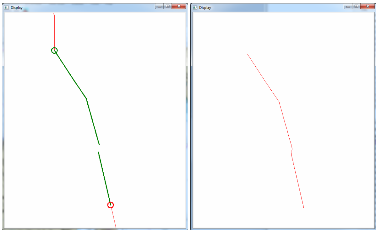
FIGURE 1. Example of a 1 Second, 3 Meter Gap That Would Have Resulted in Two Separate Files Before—Before (left) and After (right)
