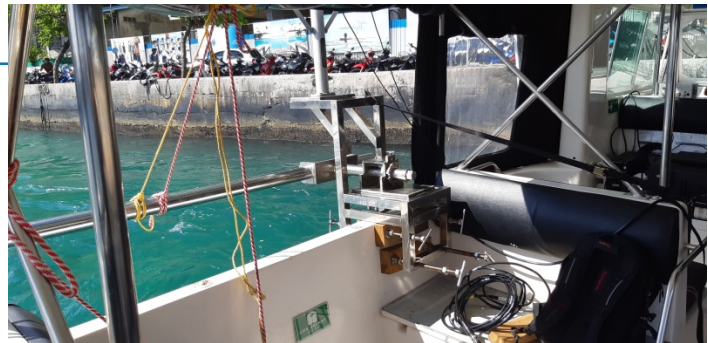
FIGURE 1. Mounting Bracket for the Norbit MBES
