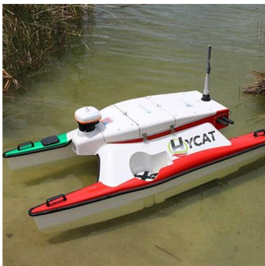
FIGURE 1. The pipeline survey was conducted using the HYCAT with a SonTek M9 HydroSurveyor.
