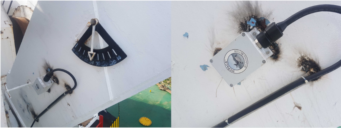
FIGURE 1. Installation of the Inclinometer
