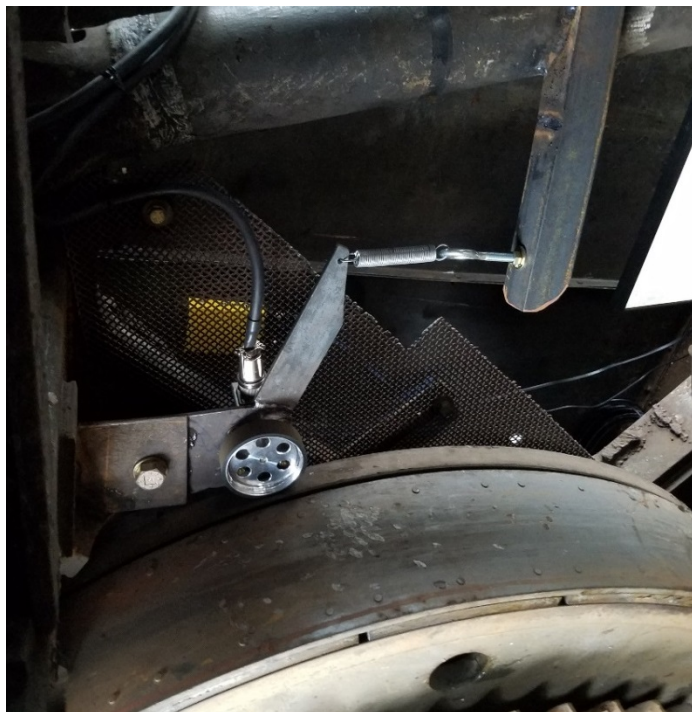
FIGURE 5. Another Possible Way to Install the Rotation Sensor
