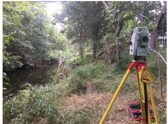
Fig. 8. Leica Total Station
