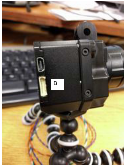
FIGURE 2. FLIR Camera Connections—Connect A to B, then modify the MAVLink connector (1) with the RS232
