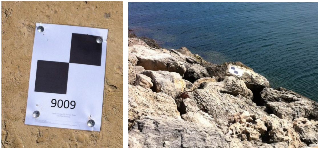
FIGURE 2. Photogrammetry Ground Control Points Established on the Breakwater Using RTK GNSS Positioning.
