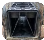
Type S Recycled Materials underdrain passes the downward loading test
