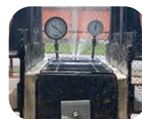
Type S Recycled Materials underdrain passes the grouted internal burst strength test
