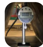
Type S Recycled Materials underdrain passes the downward loading test
