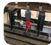
Type S Recycled Materials underdrain passes the downward loading test
