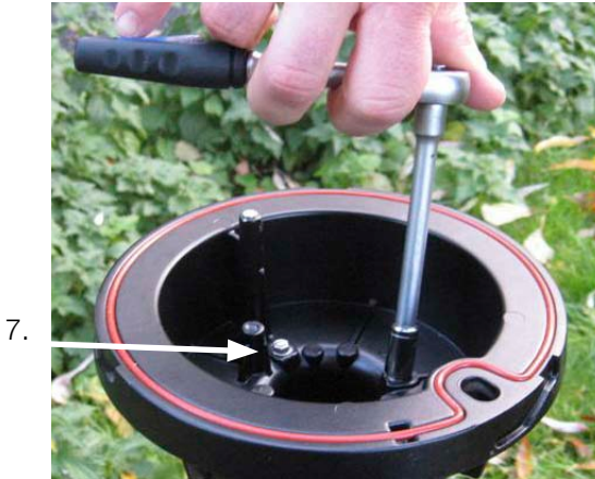
Figure 7. Tighten the Screws with a Spanner
