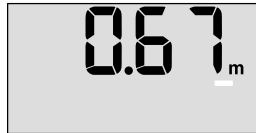
Example: Missing echo - the bar on the right hand side is flashing.
