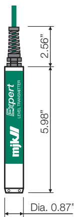
MJK Expert™ 1400 level transmitter
