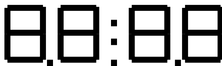
Fig. 7 LCD Display showing all segments.
