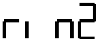
Fig. 6 Display with two rinsing cycles selected
