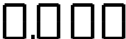
Fig. 11 Volume display after power-up.
