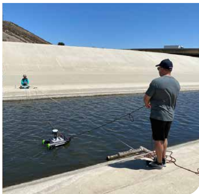
Figure 4: ADCP Streamflow gauging's with RiverSurveyor M9 and RS5. High flow conditions left, low flow conditions right.
