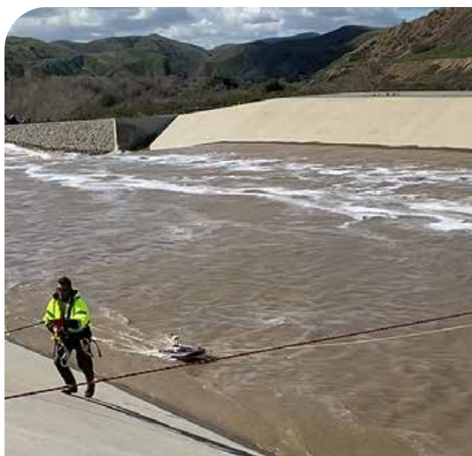
Figure 4: ADCP Streamflow gauging's with RiverSurveyor M9 and RS5. High flow conditions left, low flow conditions right.
