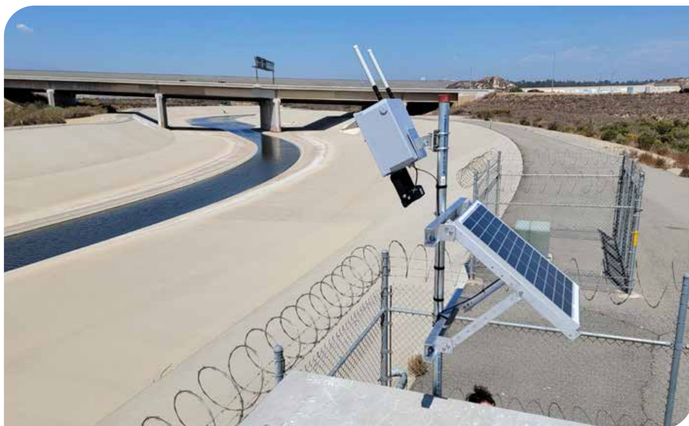
Figure 3: CVSG system installed at USGS gaging station 1107400, Santa Ana R BL Prado Dam, CA.
