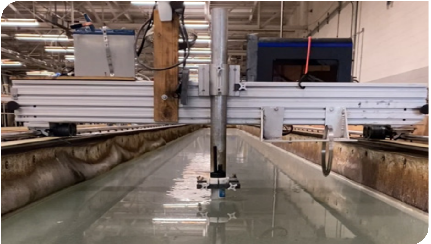
Figure 2. SonTek RS5 in the process of being verified following USGS process at the HIF.
