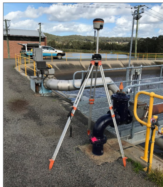
Fig. 2. Hemisphere S321 Smart Antenna.
