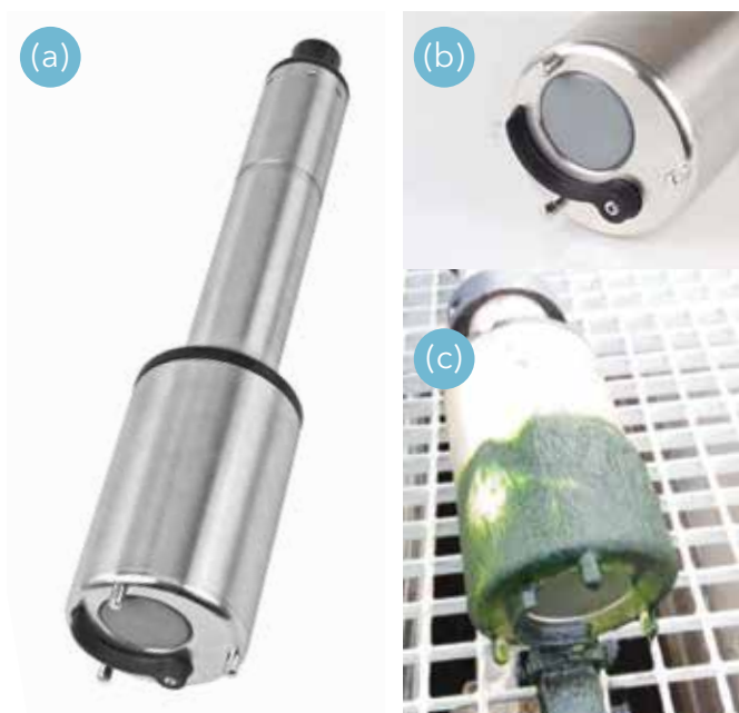
Fig. 4, WTW IFL 700 IQ sensor. (a) IFL sensor body. (b) Bottom of IFL sensor; (c) Bottom of IFL sensor even in application full of algae.
