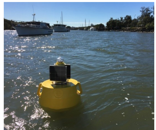
Figure 2 - Real-time water quality monitoring buoy (YSI DB600)
