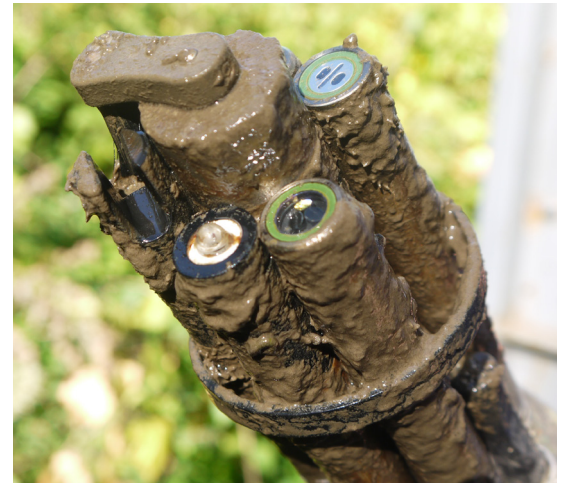
Figure 8. Effective anti-fouling using wiper
