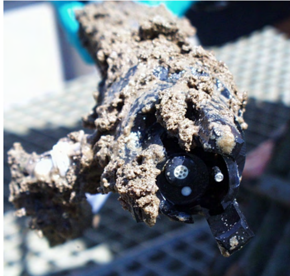
Fig 16 Left: CH cleaning head to be screwed on the VARiON system Right: Successfully keeping free the measurement electrodes during operation
