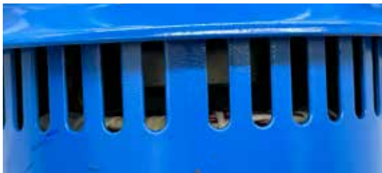
Exposed motor windings
