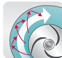
Standard impeller slams solids into the volute.
