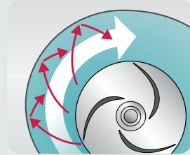
Standard impeller slams solids into the volute.
