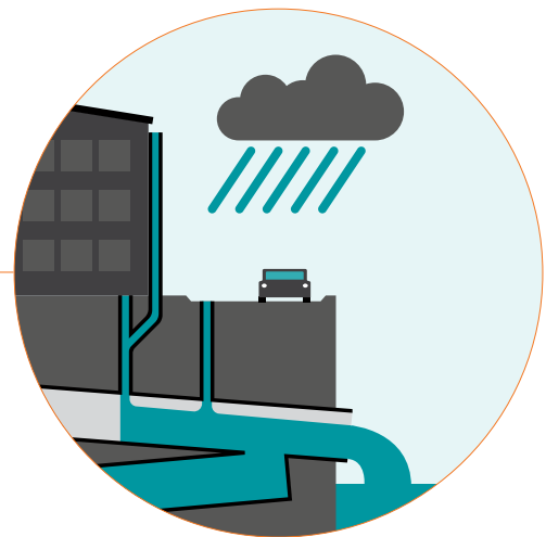
Combined Sewer Overflow (CSO)
