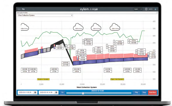
SSO/CSO Prediction and Prevention monitoring hydraulic grade lines, CSO outfall, and control gates for Evansville Water and Sewer.
