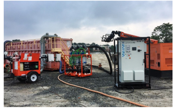
Each Flygt 2201 SH pump underwent a five-point performance test at the factory, as well as a four-point customer witness test in the assembled custom manifold in Bridgeport, New Jersey.
